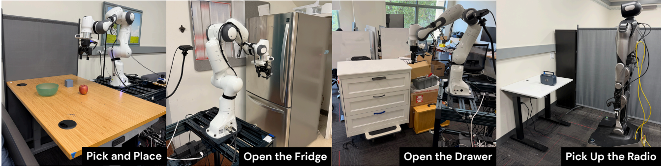
Fig. 16: Physical setups and the initial poses of the robot in completion for each task
